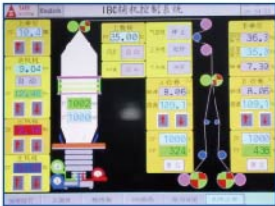
IBC 辅机控制系统 Inner bubble cooling system
